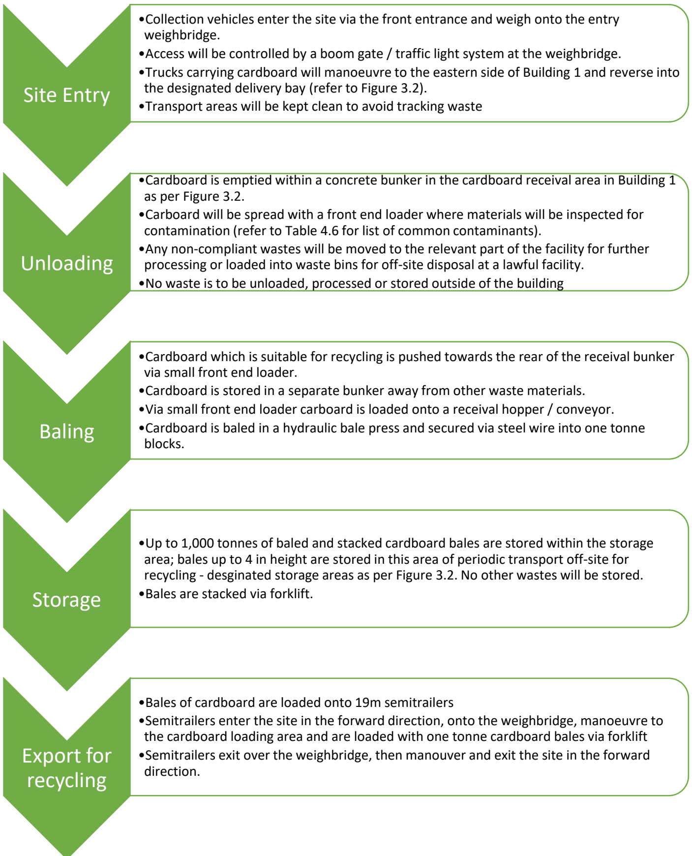
Figure 4.3. Process flow chart for the operation of the Cardboard Baling Facility.
