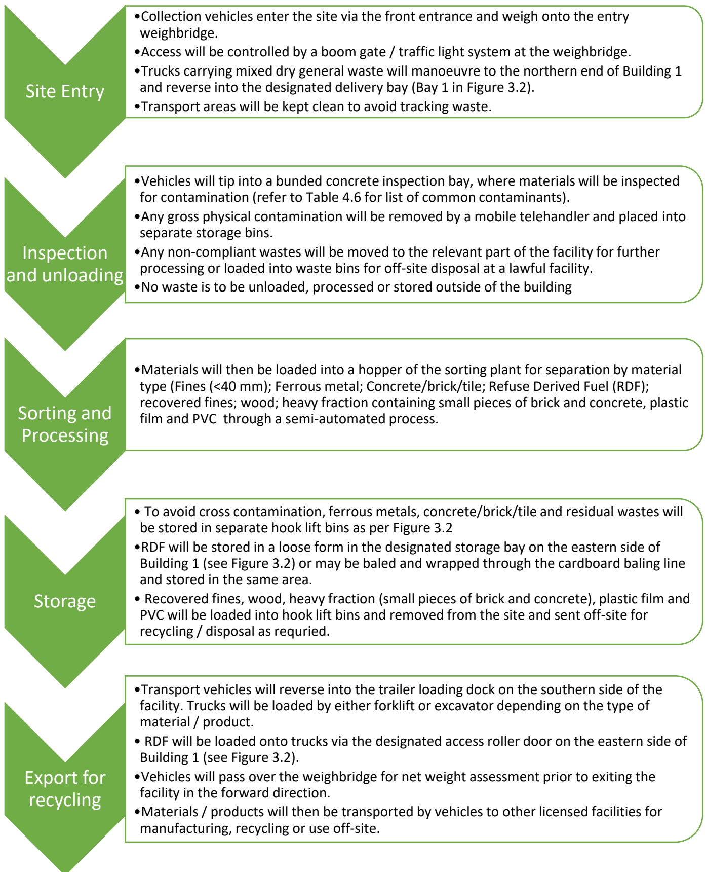
Figure 4.2. Process flow chart for the operation of the Materials Recycling Facility.
