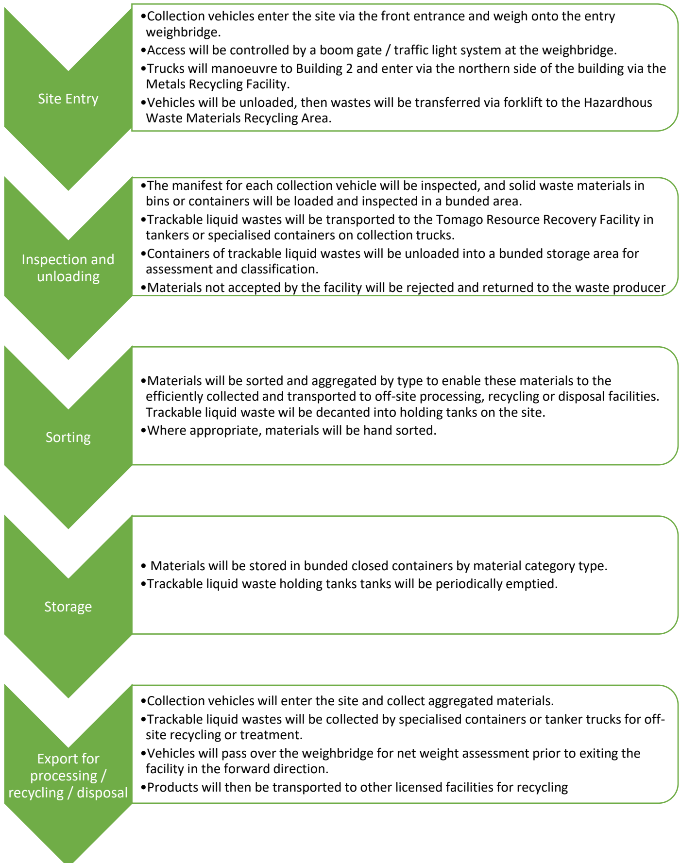
Figure 4.7. Process flow chart for the operation of the Hazardous Waste Recycling Facility.
