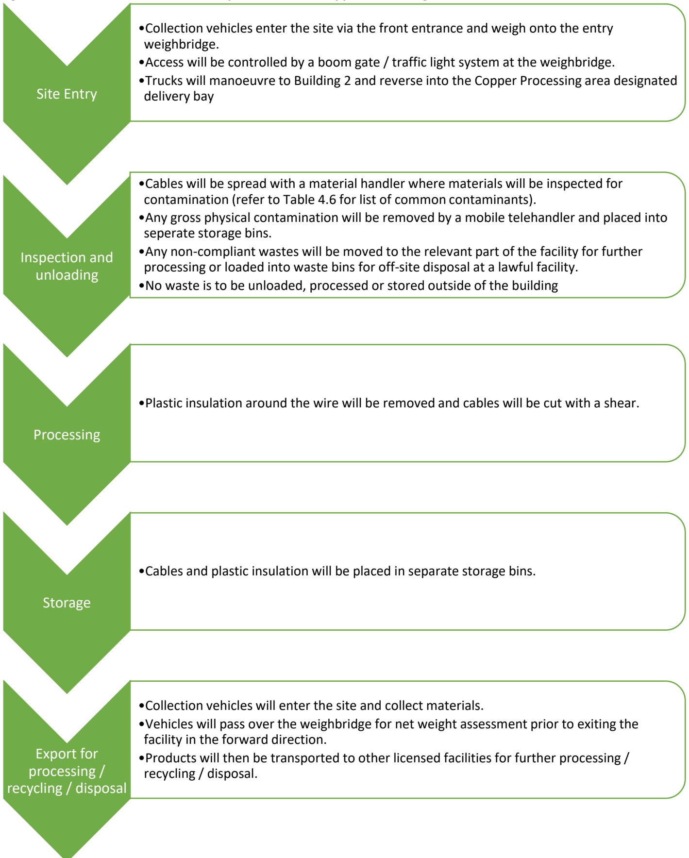
Figure 4.8. Process flow chart for the operation of the Copper Processing area.
